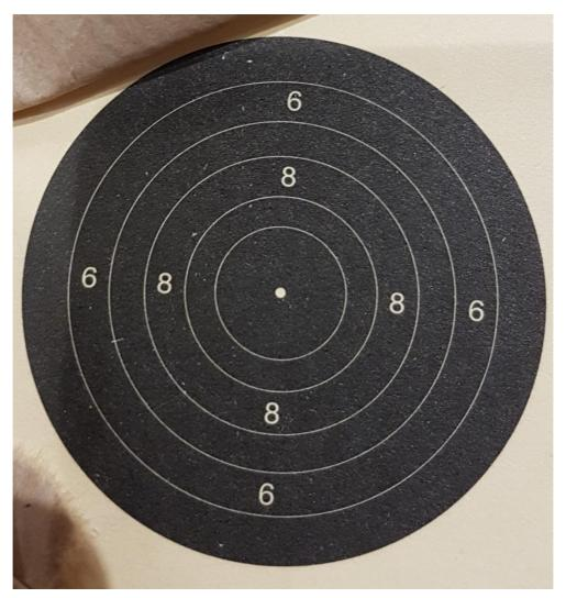
**Fault 2. Incorrect line thickness** – the lines that separate the rings are too thin. These targets may or may not *also* have Fault 1. This is difficult to identify without a correct target against which to compare, but affected cards will have the following telltales:
